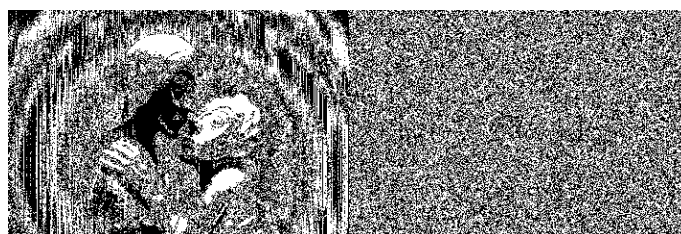
Figure 10: Embedding filter applied to Figure. 5; Steganos leaves its traces in all pixels (right).
