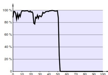
Figure 19: Embedding probability for EzStego Figure. 18; a statistical analysis of the steganography from Figure 18 shows steganographic changes.
