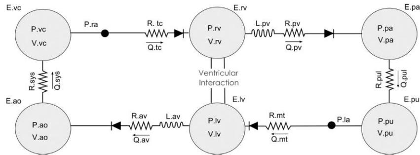
**Figure 1.** Cardiovascular system (CVS) model as an analogy of electrical circuit [30].
